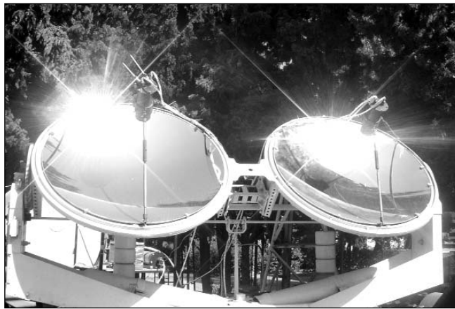
Figure 2. Solar plant with parabolic concentrator.
