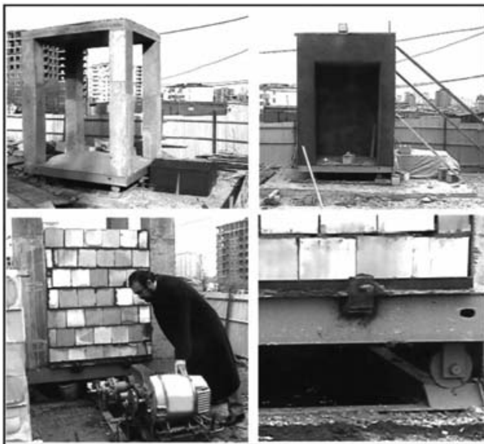
Test of model of a building from standard bricks on a small seismic platform.
