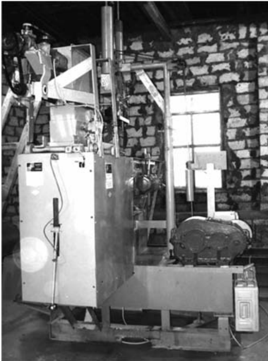
The machine tool for manufacture of aseismic building blocks.
